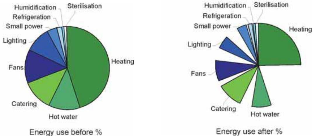
Figure 3.1 *Example of energy use in an NHS hospital before and after incorporating a carbon reduction strategy*
